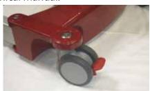
Wheels with directional lock а have brakes fitted: we therefore recommend changing only one of the rear wheels. Push down the red lever to lock the direction. To release, pull the lever up.
