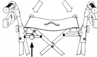
Caution! The rollator must never be used unless the locking pin (A) is properly engaged.
