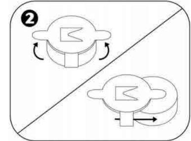
On the back of the screen unit, lift up the battery tabs and slide out the battery.
