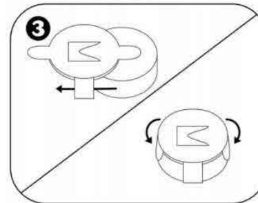
Insert a new 1.5V AG13 battery, positive side down and close the tabs.
