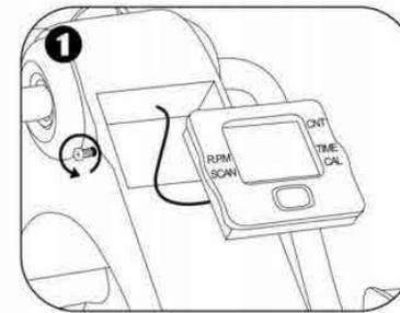
Loosen and remove the screws on each side side of the screen unit, then carefully remove the screen unit from its socket.
