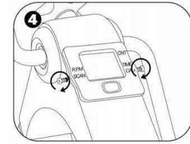
Replace the screen unit in its socket and secure with the screws.
